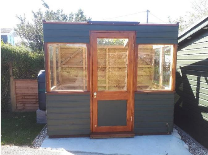
A robust but space saving timber greenhouse designed for attractiveness and longevity with less than a 3 square meter footprint (4ft x 8ft) having a heavy duty base and “tanked” floor, auto-vented roof with 4 mm toughened glass, front and side walls half glazed with 4mm glass, hardwood sills, 14mm treated shiplap back panel and base walls finished in two coat “Cuprinol Shades” of your chosen colour.
