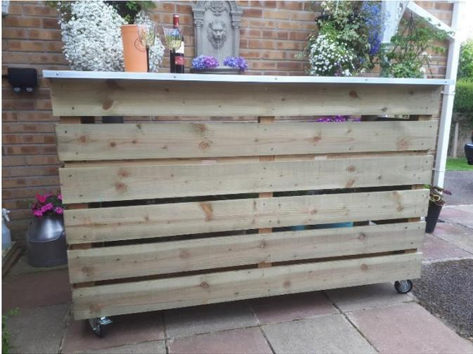
A robust mobile outside bar unit designed to withstand the elements and to be attached to similar and multiple units to form any bar length desired whilst being easily moved unit by unit.
